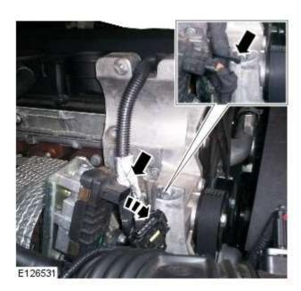
Remove the cable tie from the compressor bracket. Dis-connect the electrical connector and remove convoluted tube and high temp sleeve from Rotary Electrical Actuator breakout.
