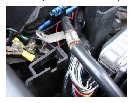
Undo the engine ECU retaining screw
