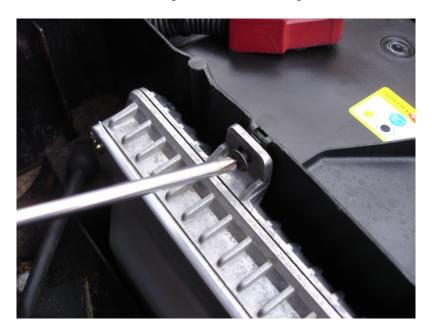
Tilt the ECU up and lift out
