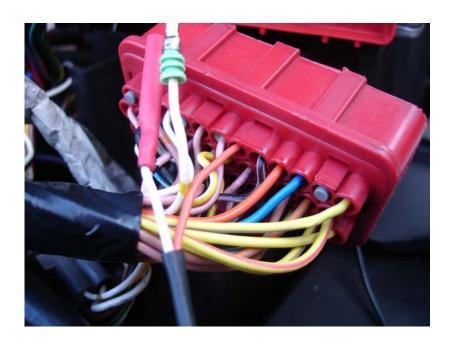
Take the lead from the **TD5 BOOSTER** with the heat shrink tubing, and push the White/Yellow cable you took out of the red plug, in to mate up with the Male connector inside.
