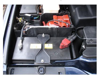
Undo the Battery lead to chassis Earth retaining nut with a 10mm Spanner.
