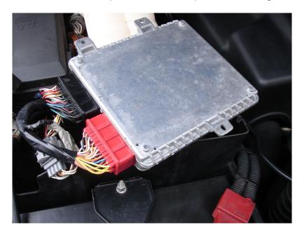
Take the red ECU plug off it's socket. There is a retaining clip on the other side of the plug, which you will need to press down to release it.
