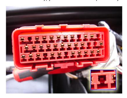
Now we need to identify the pin which needs to be removed. We are looking for Pin 6, which is located on the bottom row of the plug. As our plug is upside down, it is therefore at the top. Counting from Right to Left, starting at 1, count the pin numbers (including pins not in use) up to 6. This will be a White wire with a Yellow marking. The markings on the wire will vary depending on the year of manufacture of your vehicle. Examples of early and late model wiring is shown below.
