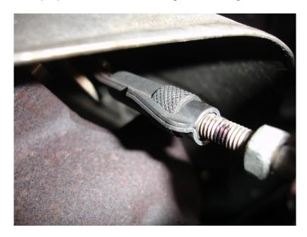
Once you have wound the adjuster up to the mark you had made on the actuator rod (approx 5 - 7mm), tighten the locknut back against the collar to prevent it from moving.
