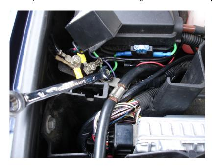
Now lift the Battery Earth cable off the chassis earth post.
