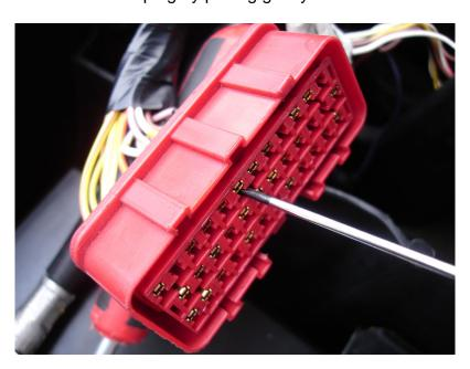
Once the connector has been released, pull it right out of it's hole.
