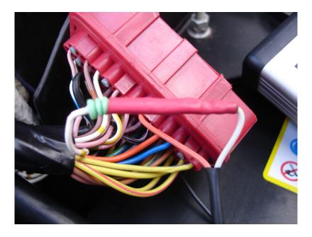
Refit the ECU, and replace the battery Earth lead onto the chassis earth post.
