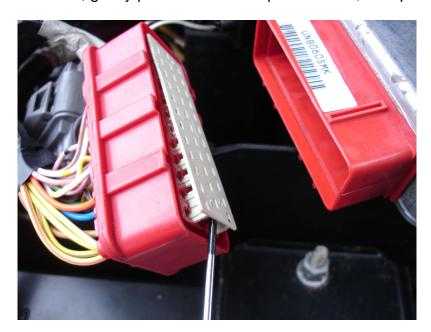
Once you've removed the plastic cover, you'll see all of the connectors in the plug. Each of these connectors are held in place with a small plastic retainer. Looking at the inset picture (connector removed for clarity) you'll see the retainer quite clearly.
