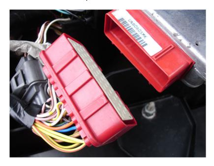
Using a small screwdriver, gently prise off the white plastic cover, to expose the terminals.
