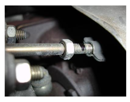
You need to turn the knurled adjuster on the actuator, in order to make your adjustment. However, it can be quite stiff so to prevent damage to the diaphragm inside the wastegate actuator, clamp the actuator rod in place with some mole grips.
