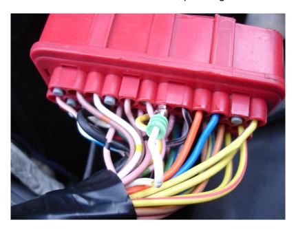
Now put the female type connector from the *TD5 BOOSTER* into this hole. Push it right in and you should hear or feel a click as it locates. Give it a gentle tug, and it should stay put.
